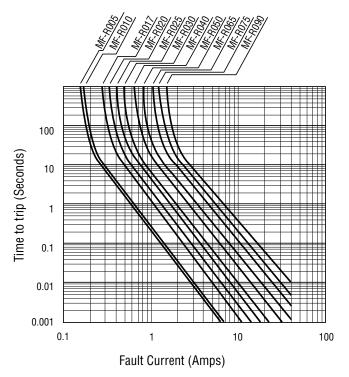
The Time to Trip curves represent typical performance of a device in a simulated application environment. Actual performance in specific customer applications may differ from these values due to the influence of other variables.
