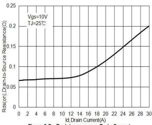
Figure 3.On-Resistance versus Drain Current
