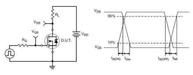
Resistive Switching Test Circuit
