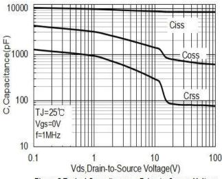
Figure 5.Typical Capacitance vs.Drian-to-Source Voltage
