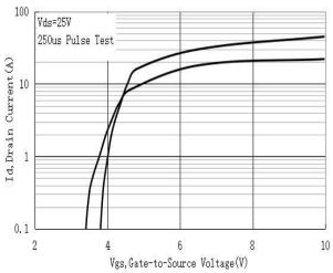
Figure 2. Typical Transfer Characteristics
