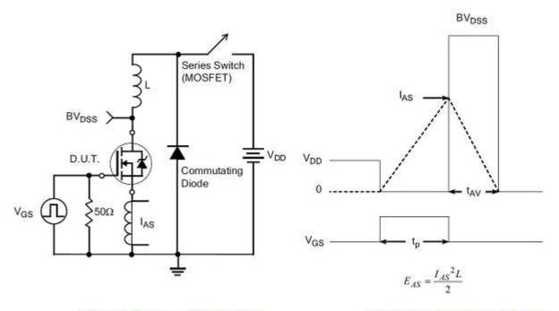
Unclamped Inductive Switching Test Circuit
