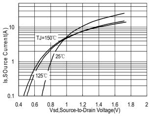
Figure 4.Diode Forward Voltage versus Current
