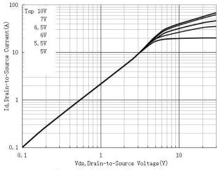
Figure 1. Typical Output Characteristics
