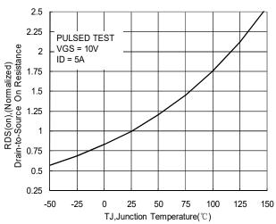
Figure 8.On-Resistance Variation with Temperature
