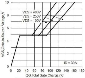
Figure 6. Typical Gate Charge vs. Vgs
