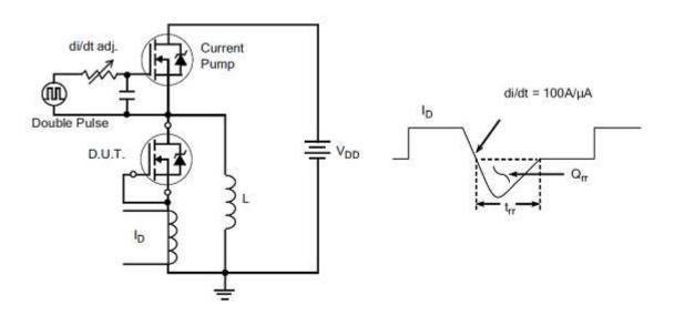
Diode Reverse Recovery Test Circuit
