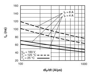
Fig. 5 - Typical Reverse Recovery Time vs. dl<sub>F</sub>/dt
