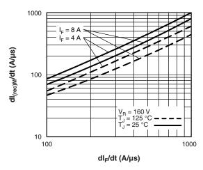
Fig. 8 - Typical dI<sub>(rec)M</sub>/dt vs. dI<sub>F</sub>/dt
