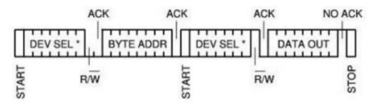
IIC read timing diagram
