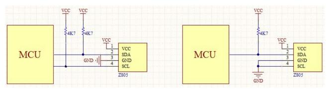
IIC typical application circuit
