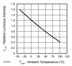
Figure 8. Relative Luminous Intensity vs. Ambient Temperature
