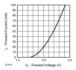
Figure 4. Forward Current vs. Forward Voltage
