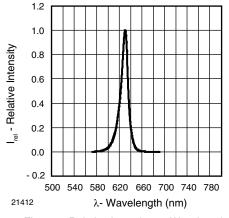
Figure 3. Relative Intensity vs. Wavelength
