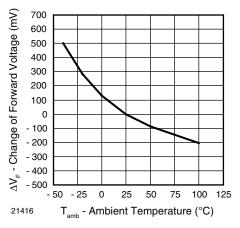
Figure 7. Change of Forward Voltage vs. Ambient Temperature
