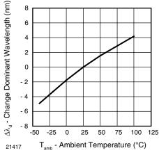
Figure 9. Change of Dominant Wavelength vs. Ambient Temperature
