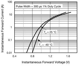
Fig. 3 - Typical Instantaneous Forward Characteristics
