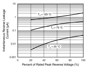
Fig. 4 - Typical Reverse Leakage Characteristics
