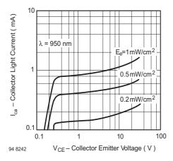
Figure 5. Collector Light Current vs. Collector Emitter Voltage
