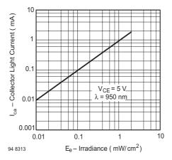
Figure 4. Collector Light Current vs. Irradiance
