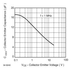
Figure 6. Collector Emitter Capacitance vs. Collector Emitter Voltage
