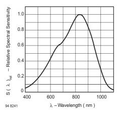
Figure 8. Relative Spectral Sensitivity vs. Wavelength
