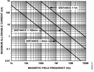
Figure 27. Maximum Allowable Current for Various Current-to-ADM3053 Spacings
