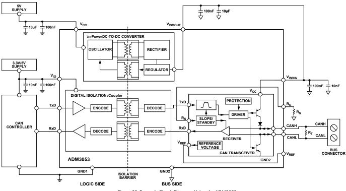
Figure 32. Example Circuit Diagram Using the ADM3053
