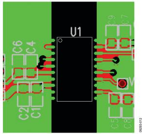
Figure 28. Recommended PCB Layout
