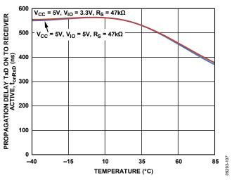
Figure 12. Propagation Delay from TxD On to Receiver Active vs. Temperature
