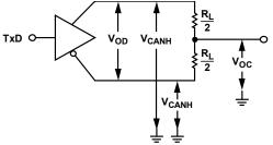
Figure 22. Driver Voltage Measurement
