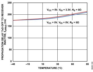
Figure 13. Propagation Delay from TxD Off to Receiver Inactive vs. Temperature
