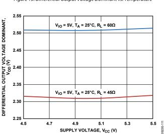
Figure 16. Differential Output Voltage Dominant vs. Supply Voltage,  $V_{CC}$
