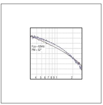
Figure 3. MAX17501G Full-Load Bode Plot ( $V_{IN} = 24V$ )
