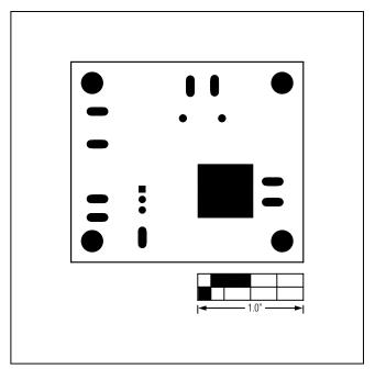
Figure 11. MAX17501G EV Kit PCB Layout—Bottom Solder Mask
