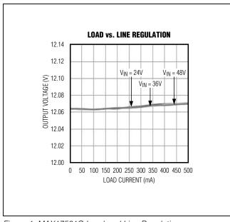
Figure 1. MAX17501G Load and Line Regulation
