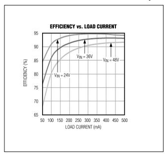
Figure 2. MAX17501G Efficiency
