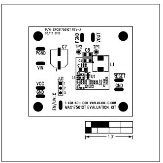
Figure 7. MAX17501G EV Kit Component Placement Guide—Component Side
