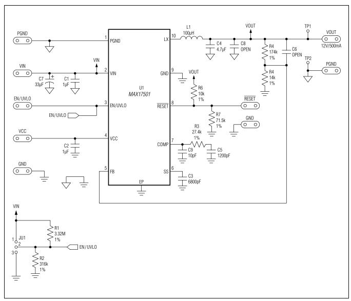
Figure 6. MAX17501G EV Kit Schematic
