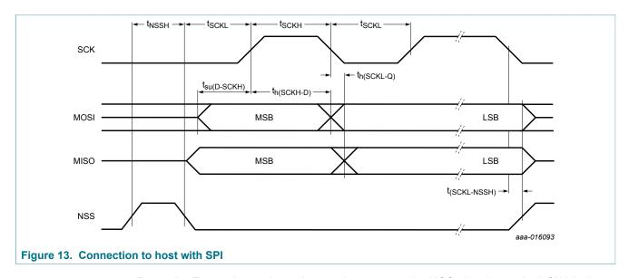
**Remark:** To send more bytes in one data stream, the NSS signal must be LOW during the send process. To send more than one data stream, the NSS signal must be HIGH between each data stream.
