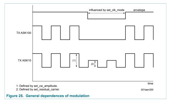
Note: When changing the continuous carrier amplitude, the residual carrier amplitude also changes, while the modulation index remains the same.
