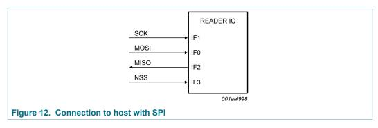
The CLRC663 acts as a slave during the SPI communication. The SPI clock SCK has to be generated by the master. Data communication from the master to the slave uses the Line MOSI. Line MISO is used to send data back from the CLRC663 to the master.
