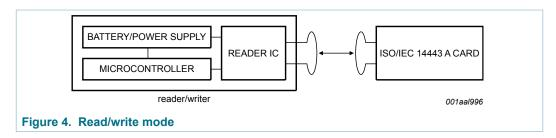
A typical system using the CLRC663 is using a microcontroller to implement the higher levels of the contactless communication protocol and a power supply (battery or external supply).
