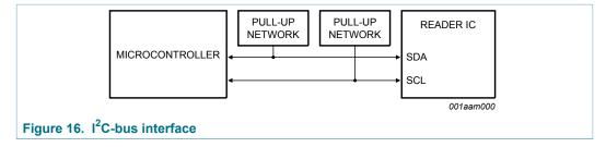
The voltage level on the I2C pins is not allowed to be higher than PVDD.
