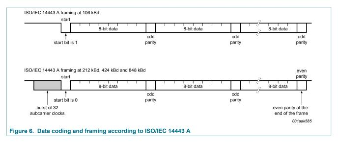
The internal CRC coprocessor calculates the CRC value based on ISO/IEC 14443 A part 3 and handles parity generation internally according to the transfer speed.
