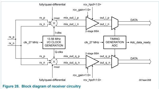
The receiver can also be operated in a single ended mode. In this case, the Rcv RX single bit has to be set. In the single ended mode, the two receiver pins RXP and RXN need to be connected together and will provide a single ended signal to the receiver circuitry.
