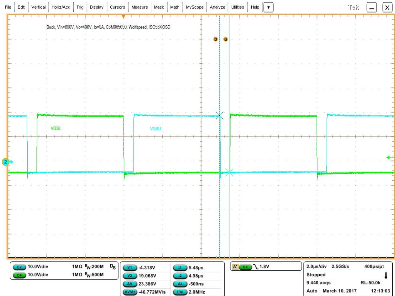
Figure 6. Gate-Source Driver Voltage
