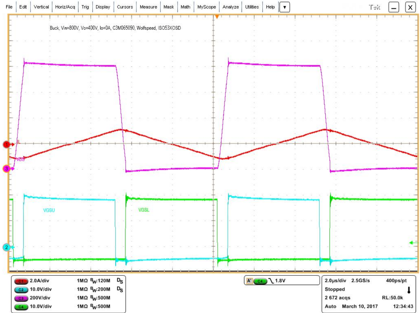
Figure 9. Inductor Current (Red), Drain-Source (Pink) and Gate-Source Drive Voltages (Blue and Green) at 800-V Input, 0-A Output
