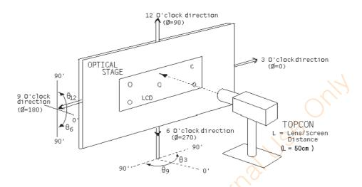
**Figure 2** Response Time Testing
