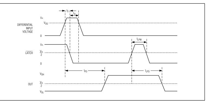
Figure 2. MAX941 Timing Diagram with Latch Operator
