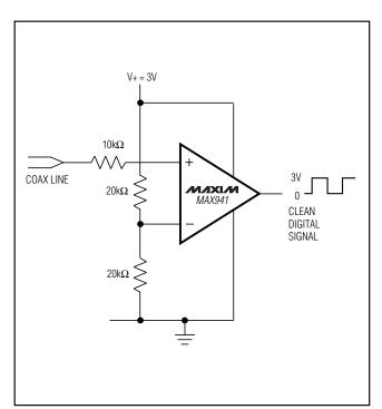
Figure 6. Line Transceiver Application
