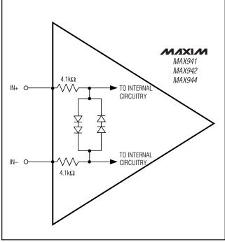
Figure 3. Input Stage Circuitry
