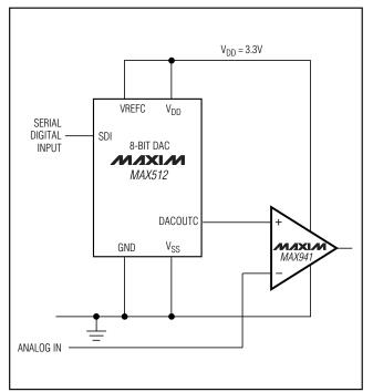
Figure 5. 3.3V Digitally Controlled Threshold Detector
