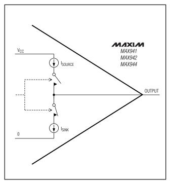
Figure 4. Output Stage Circuitry
