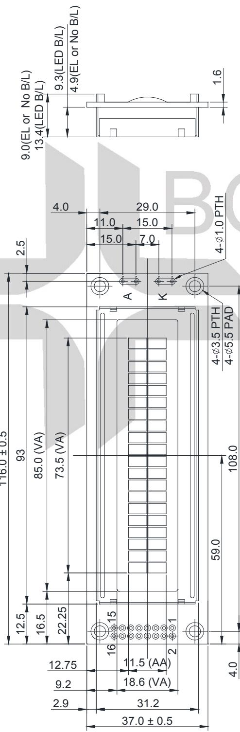
The non-specified tolerance of dimension is  $\pm 0.3$  mm .
