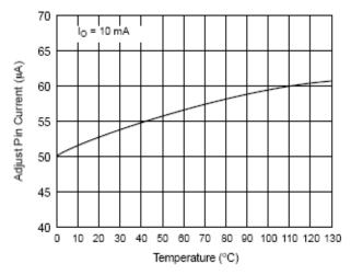
Figure 5. Adjust Pin Current vs Temperature
