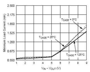
Figure 4. Minimum Load Current
