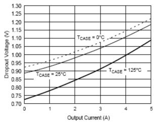
Figure 1. Dropout Voltage vs Output Current
