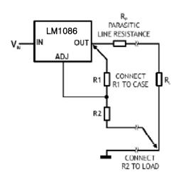
True remote sheet specification it is not possible to provide, because the LM1086 is a three terminal device. The resistance of the wire connecting the regulator to the load will limit the load regulation.
