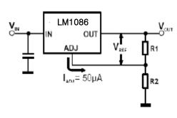
The LM1086 series develops a 1.25V reference voltage between the output and the adjust terminal. Placing a resistor between these two terminals causes a constant current to flow through R1 and down throuth R2 to set the overall output voltage.
