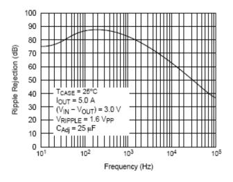
Figure 9. Ripple Rejection vs. Frequency (Adjustable Versions)
