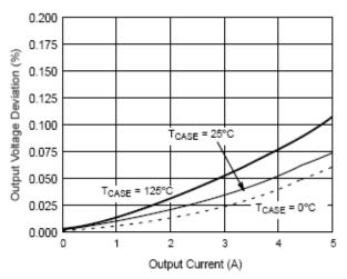
Figure 3. Load Regulation vs. Output Current
