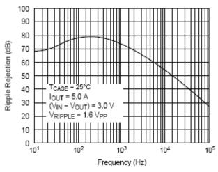
Figure 6. Ripple Rejection vs. Frequency (Fixed Versions)
