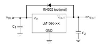
Figure 11. Protection Diode Scheme for Fixed Output Regulators
