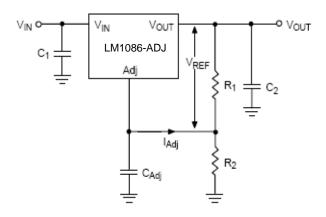
Figure 10. Resistor Divider Scheme for the Adjustable Version
