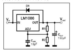
Unlike older regulators, the LM1086 family does not need any protection diodies between the adjustment pin and the output and from the output tu the input to prevent over-stressing the di Internal resistors are limiting the internal current paths on the LM1086 adjustment pin, therfore even with capacitors on the adjustment pin no protection diode is needed to ensure device safety under short-circuit conditions.
