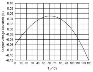
Figure 2. Reference Voltage vs Temperature
