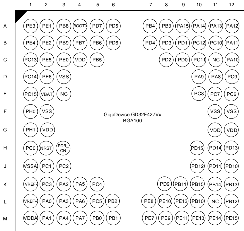
Figure 2-3. GD32F427Vx BGA100 pinouts
