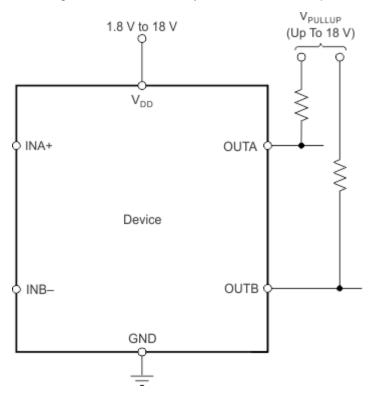
Figure 16. Interfacing to Voltages Other Than  $V_{\text{DD}}$
