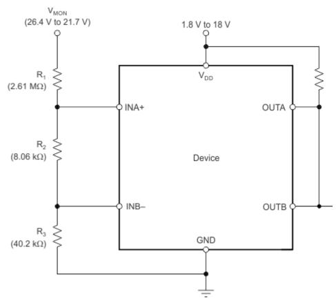
NOTE: The inputs can monitor a voltage higher than V<sub>DD</sub>max with the use of an external resistor divider network.
