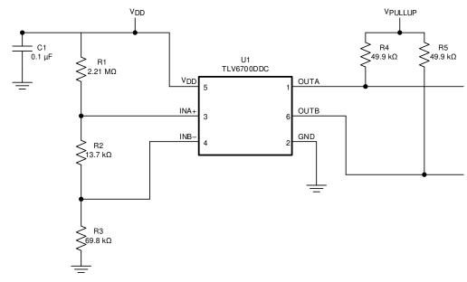
Figure 19. Typical Application Schematic
