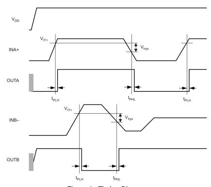
Figure 1. Timing Diagram
