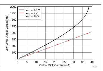
Figure 9. Output Voltage Low (V<sub>OL</sub>) vs Output Sink Current (-40°C)
