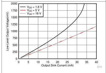
Figure 10. Output Voltage Low ( $V_{OL}$ ) vs Output Sink Current (0°C)
