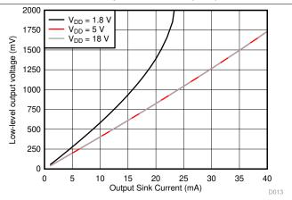
Figure 13. Output Voltage Low (V<sub>OL</sub>) vs Output Sink Current (125°C)
