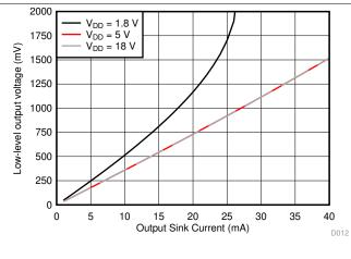
Figure 12. Output Voltage Low (V<sub>OL</sub>) vs Output Sink Current (85°C)
