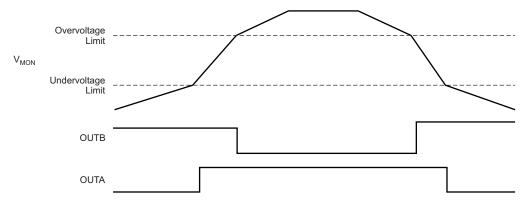
Figure 15. Window Comparator Timing Diagram
