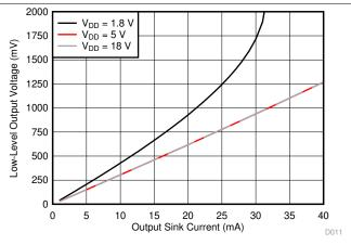
Figure 11. Output Voltage Low (V<sub>OL</sub>) vs Output Sink Current (25°C)
