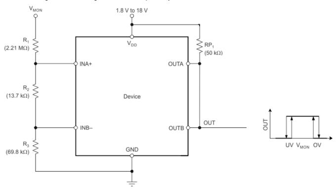
Figure 14. Window Comparator Block Diagram
