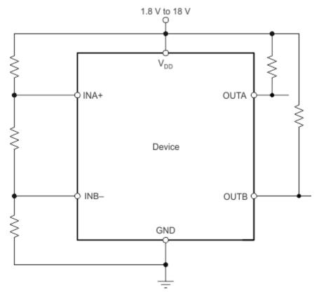
Figure 17. Monitoring the Same Voltage as V<sub>DD</sub>
