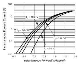
Fig. 3 - Typical Instantaneous Forward Characteristics
