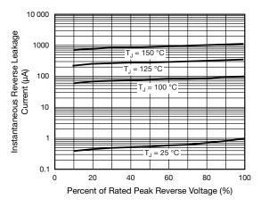
Fig. 4 - Typical Reverse Leakage Characteristics
