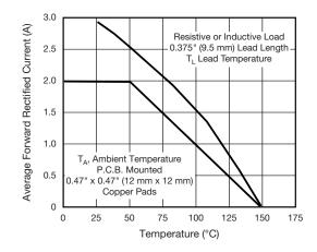
Fig. 1 - Maximum Forward Current Derating Curves
