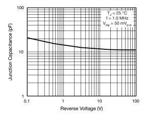
Fig. 6 - Typical Junction Capacitance
