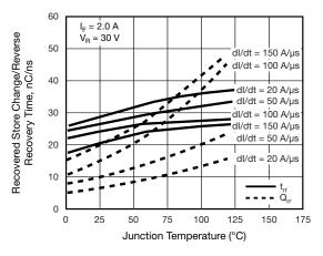
Fig. 5 - Reverse Switching Charateristics
