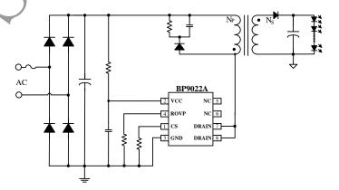
Figure 1. Typical application circuit for BP9022A
