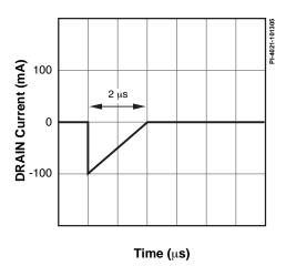
Figure 10. Peak Negative Pulsed DRAIN Current Waveform.
