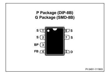
Figure 3. Pin Configuration.
