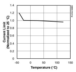
Figure 13. Current Limit vs. Temperature.
