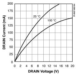
Figure 16. Output Characteristics.
