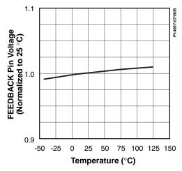
Figure 14. FEEDBACK Pin Voltage vs. Temperature.
