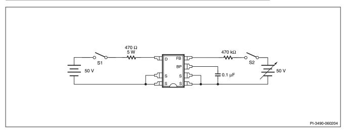
Figure 7. General Test Circuit.
