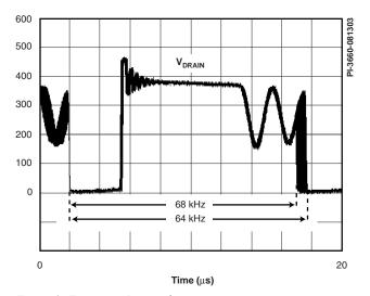
Figure 4. Frequency Jitter at fosc.
