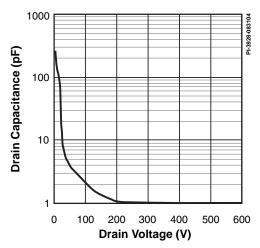
Figure 17.  $C_{OSS}$  vs. Drain Voltage.
