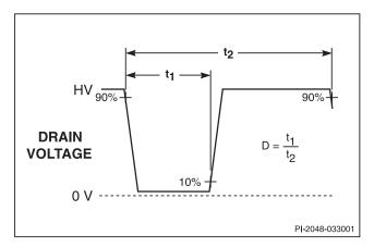
DC<sub>MAX</sub> (internal signal)
