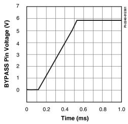
Figure 15. BYPASS Pin Start-up Waveform.
