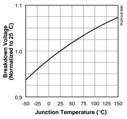
Figure 11. Breakdown vs. Temperature.
