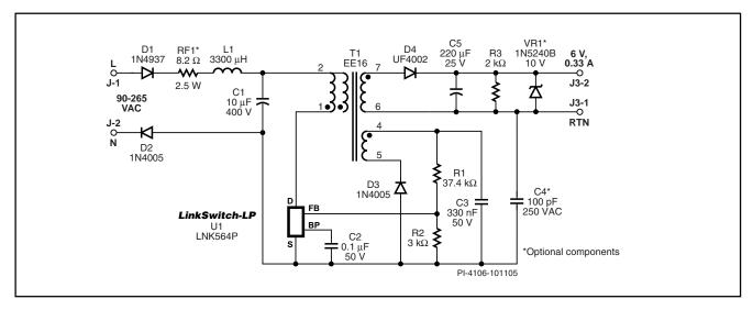
Figure 5. 6 V, 330 mA CV/CC Linear Replacement Power Supply.
