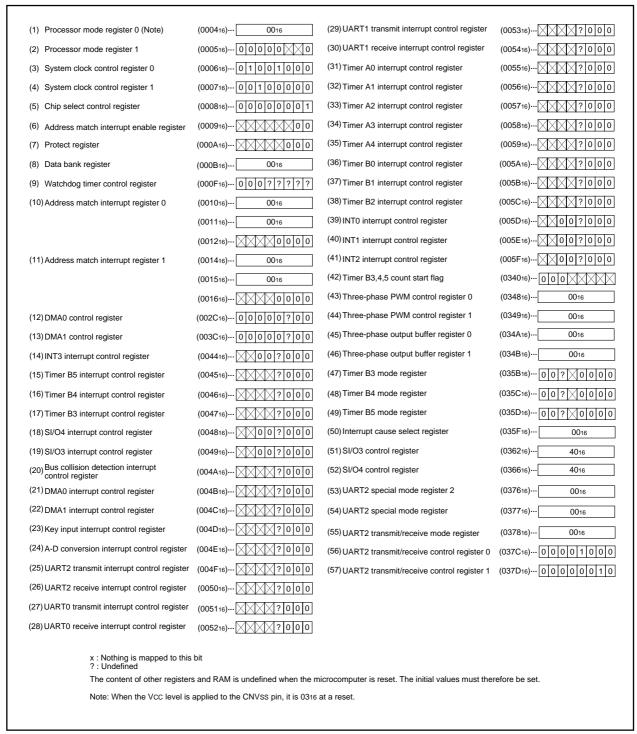
Figure 1.6.3. Device's internal status after a reset is cleared
