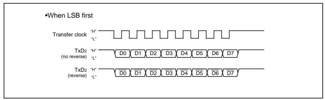
Figure 1.19.14. Serial data logic switch timing
