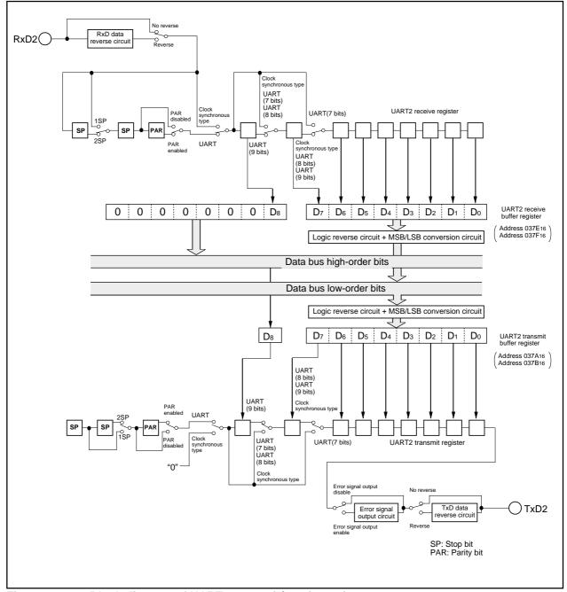
Figure 1.19.3. Block diagram of UART2 transmit/receive unit
