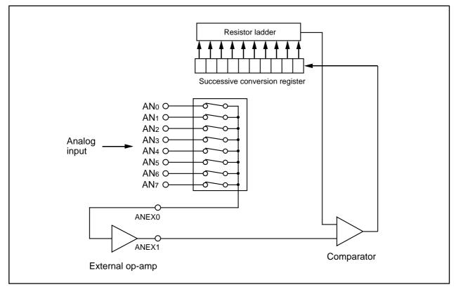
Figure 1.20.9. Example of external op-amp connection mode
