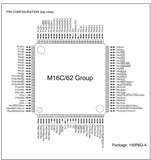
Figure 1.1.2. Pin configuration (top view)
