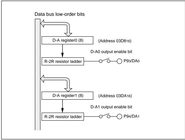
Figure 1.21.1. Block diagram of D-A converter
