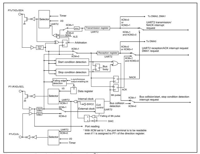
Figure 1.19.30. Functional block diagram for I<sup>2</sup>C mode
