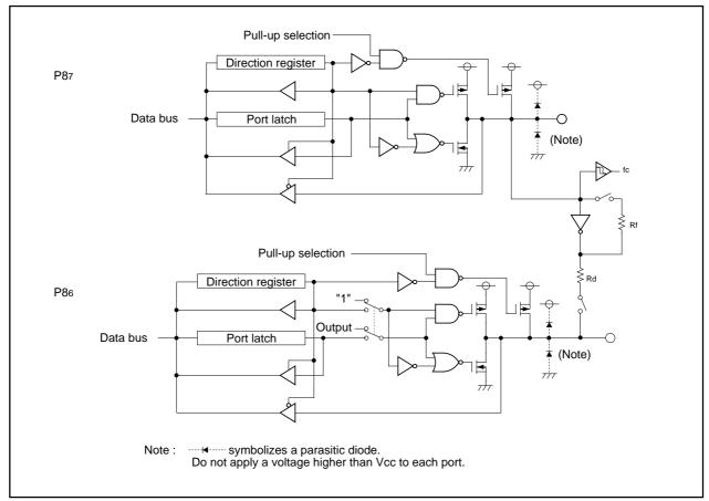
Figure 1.23.4. Programmable I/O ports (4)
