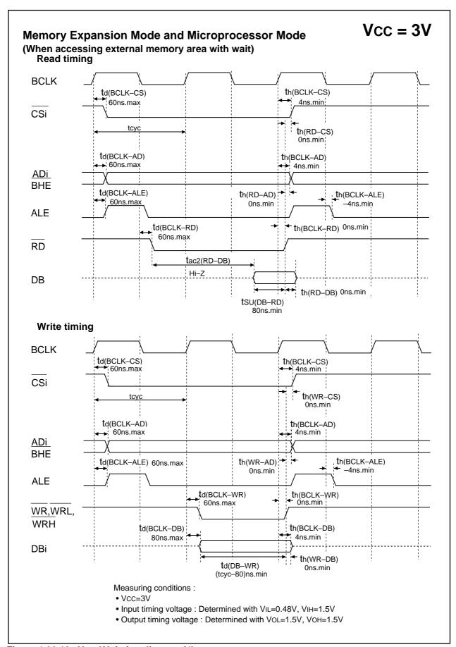
Figure 1.26.10. Vcc=3V timing diagram (4)
