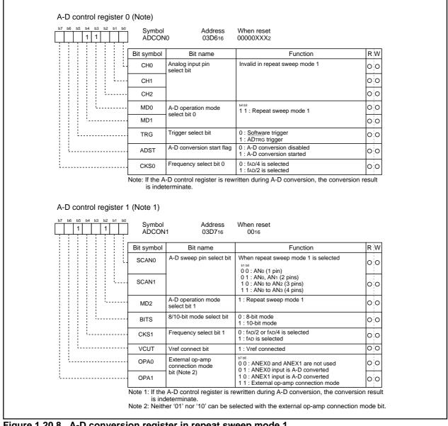
Figure 1.20.8. A-D conversion register in repeat sweep mode 1
