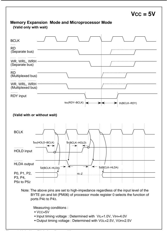
Figure 1.26.3. Vcc=5V timing diagram (2)
