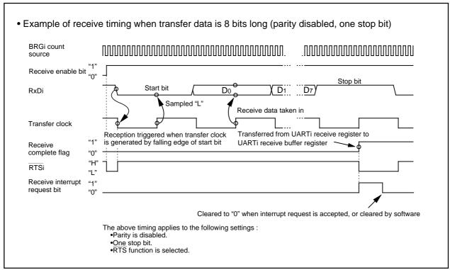
Figure 1.19.18. Typical receive timing in UART mode
