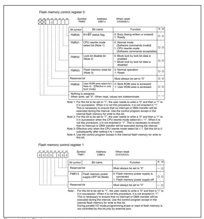
Figure 1.29.1. Flash memory control registers
