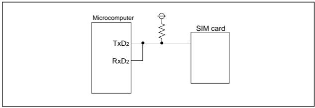
Figure 1.19.25. Connecting the SIM interface
