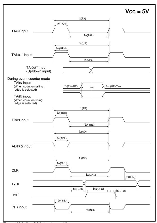
Figure 1.26.2. Vcc=5V timing diagram (1)
