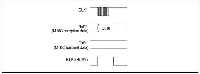
Figure 1.31.5. Timing for clearing the status register
