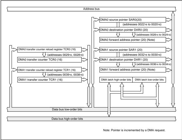
Figure 1.16.1. Block diagram of DMAC
