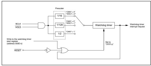
Figure 1.15.1. Block diagram of watchdog timer
