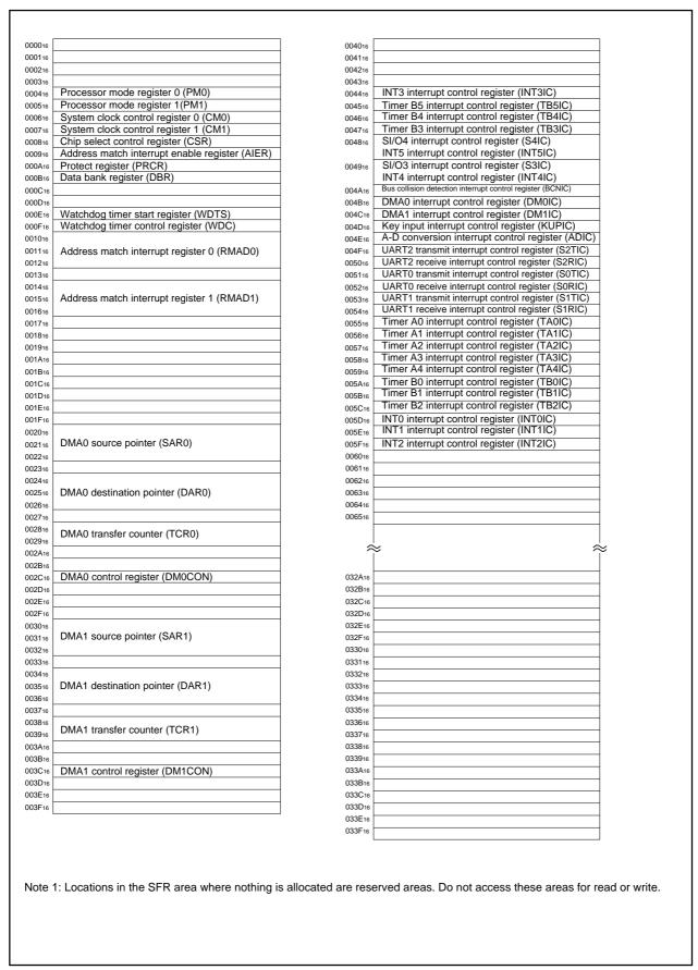
Figure 1.7.1. Location of peripheral unit control registers (1)
