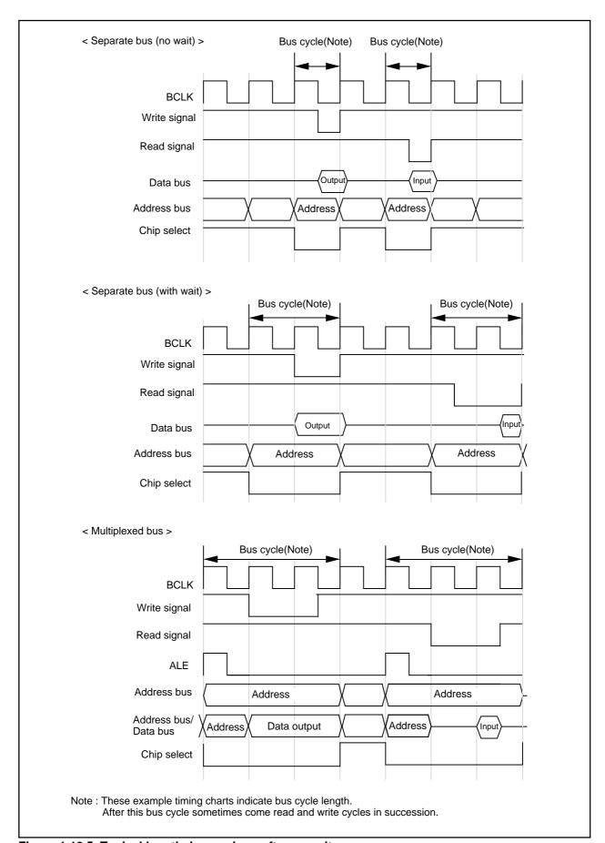
Figure 1.12.5. Typical bus timings using software wait
