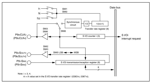
Figure 1.19.31. S I/O3, 4 block diagram
