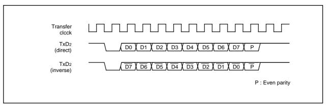
Figure 1.19.24. SIM interface format
