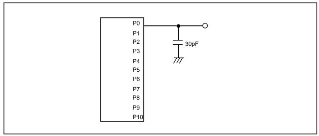
Figure 1.26.1. Port P0 to P10 measurement circuit
