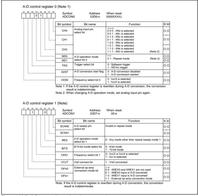
Figure 1.20.5. A-D conversion register in repeat mode
