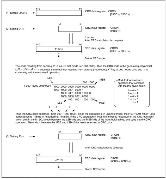
Figure 1.22.3. Calculation example using the CRC calculation circuit
