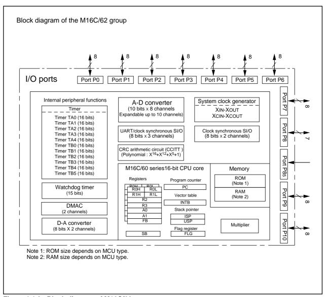
Figure 1.1.3. Block diagram of M16C/62 group
