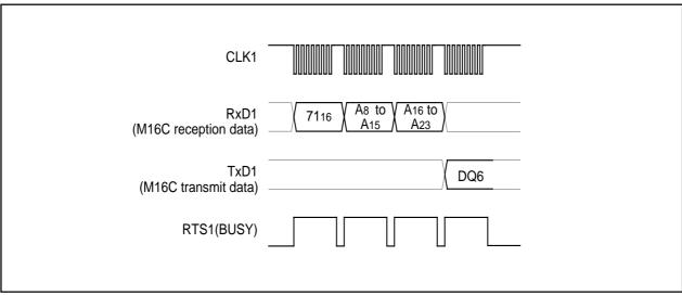
Figure 1.31.10. Timing for reading lock bit status
