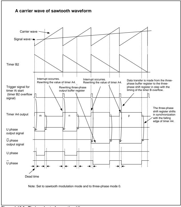
Figure 1.18.9. Timing chart of operation (4)
