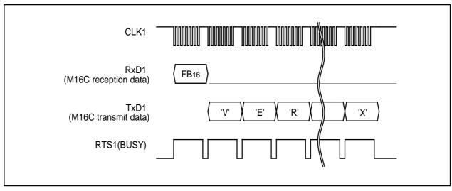
Figure 1.31.14. Timing for version information output
