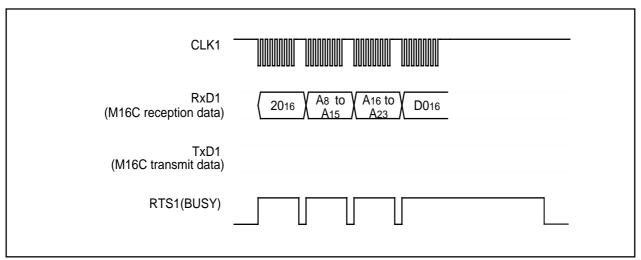
Figure 1.31.7. Timing for block erasing
