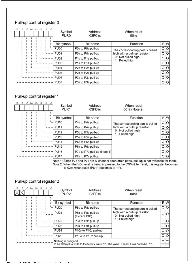
Figure 1.23.8. Pull-up control register
