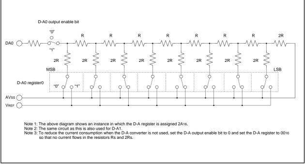
Figure 1.21.3. D-A converter equivalent circuit
