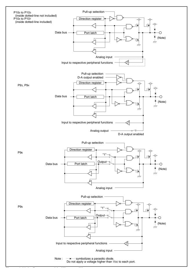
Figure 1.23.3. Programmable I/O ports (3)
