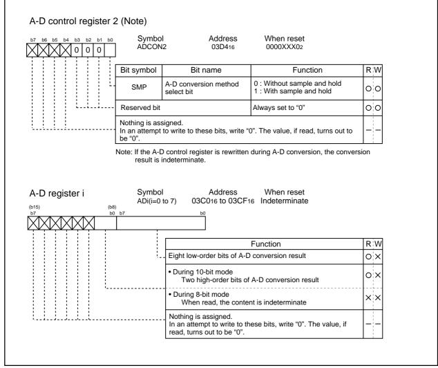
Figure 1.20.3. A-D converter-related registers (2)
