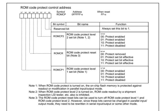
Figure 1.29.9. ROM code protect control address
