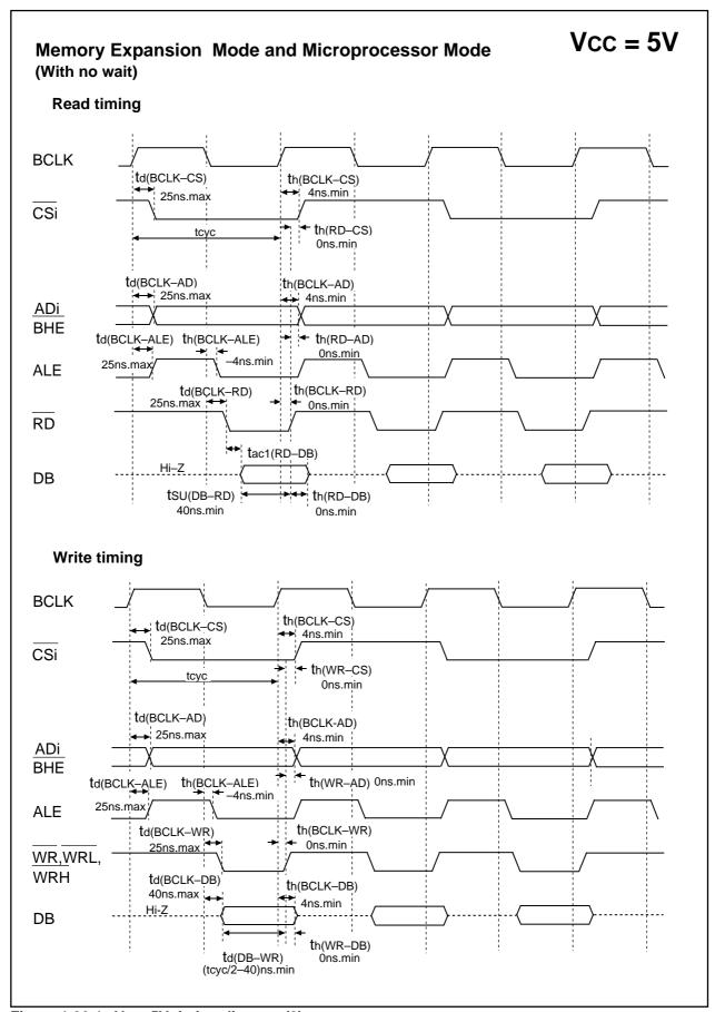
Figure 1.26.4. Vcc=5V timing diagram (3)
