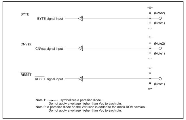
Figure 1.23.5. I/O pins
