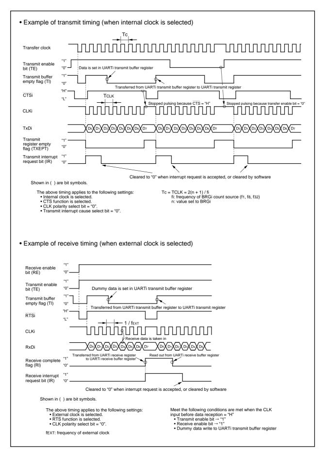
Figure 1.19.10. Typical transmit/receive timings in clock synchronous serial I/O mode
