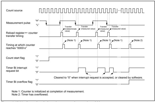
Figure 1.17.21. Operation timing when measuring a pulse width
