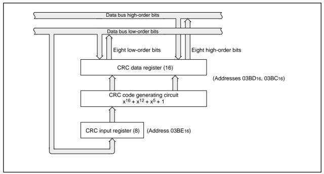
Figure 1.22.1. Block diagram of CRC circuit
