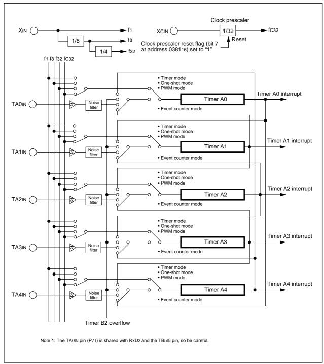
Figure 1.17.1. Timer A block diagram
