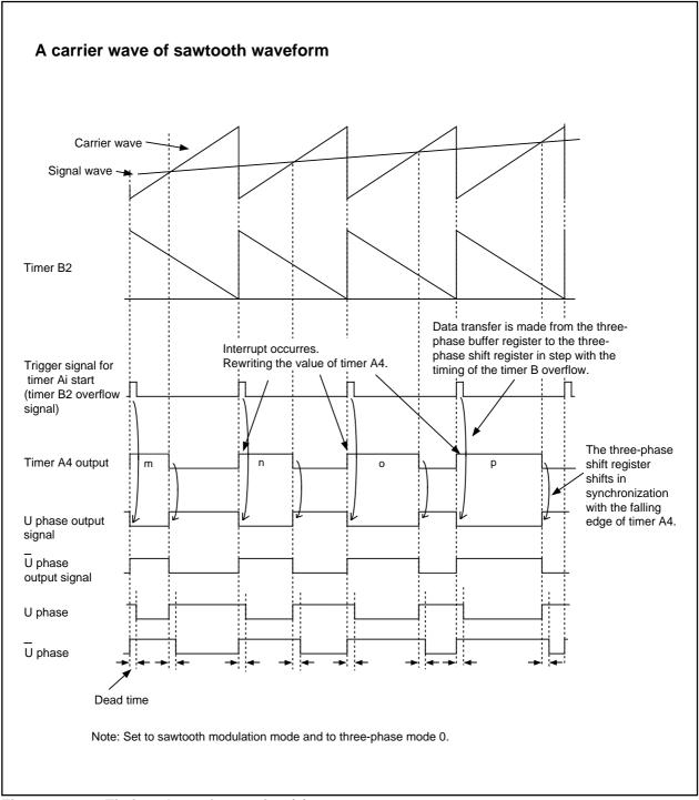
Figure 1.18.8. Timing chart of operation (3)
