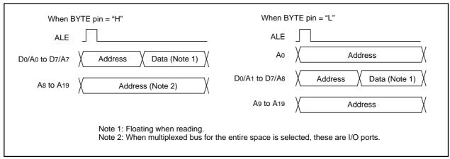
Figure 1.12.2. ALE signal and address/data bus
