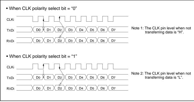
Figure 1.19.11. Polarity of transfer clock
