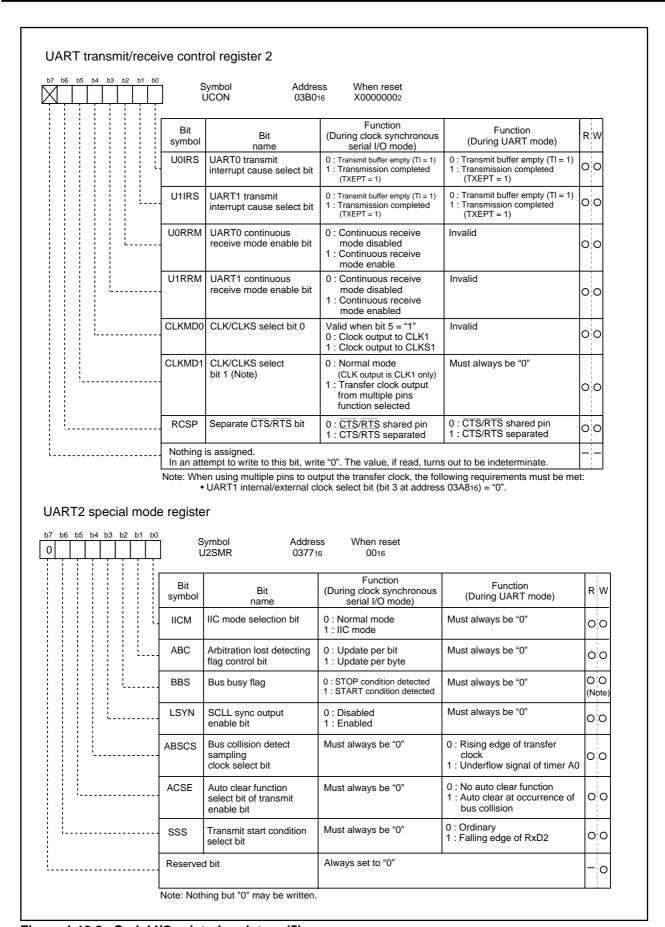
Figure 1.19.8. Serial I/O-related registers (5)
