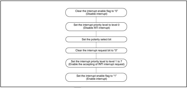
Figure 1.14.13. Switching condition of INT interrupt request
