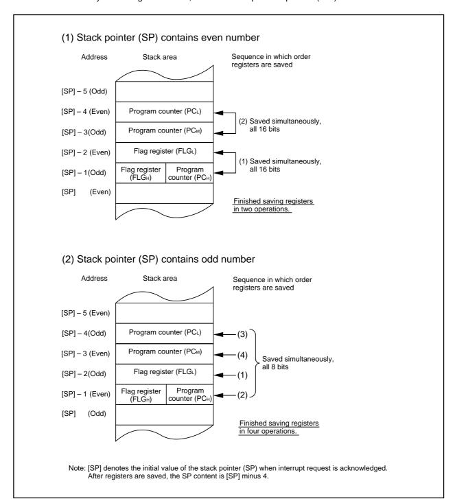
Figure 1.14.7. Operation of saving registers
