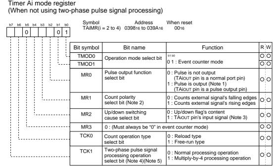
Note 1: The settings of the corresponding port register and port direction register are invalid.
