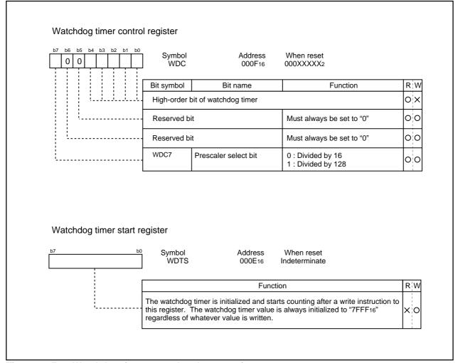
Figure 1.15.2. Watchdog timer control and start registers
