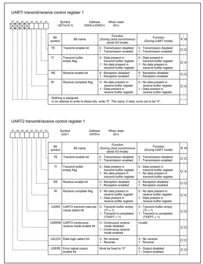
Figure 1.19.7. Serial I/O-related registers (4)
