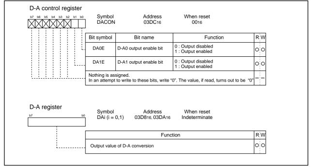
Figure 1.21.2. D-A control register
