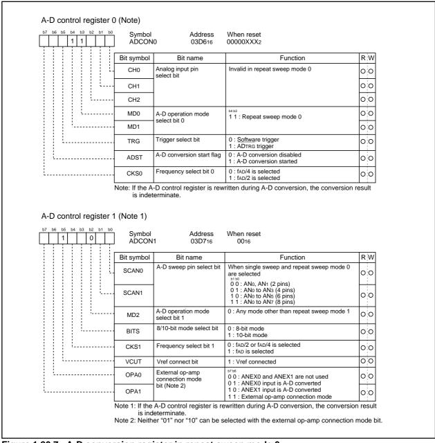
Figure 1.20.7. A-D conversion register in repeat sweep mode 0
