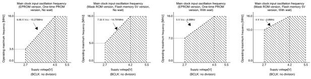
Note 5: Execute case without wait, program / erase of flash memory by Vcc=4.2V to 5.5V and  $f(BCLK) \le 6.25$  MHz. Execute case with wait, program / erase of flash memory by Vcc=4.2V to 5.5V and  $f(BCLK) \le 12.5$  MHz.
