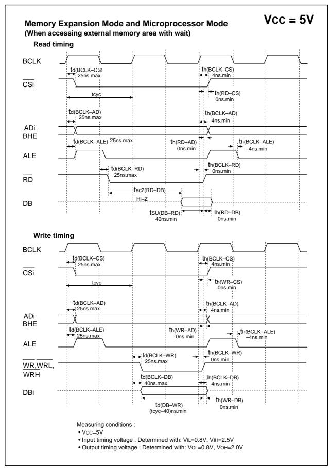
Figure 1.26.5. Vcc=5V timing diagram (4)
