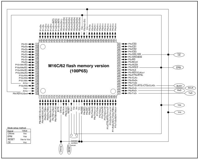
Figure 1.31.1. Pin connections for serial I/O mode (1)
