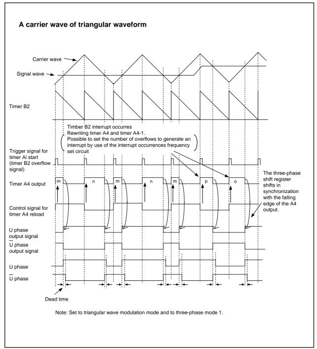
Figure 1.18.6. Timing chart of operation (1)
