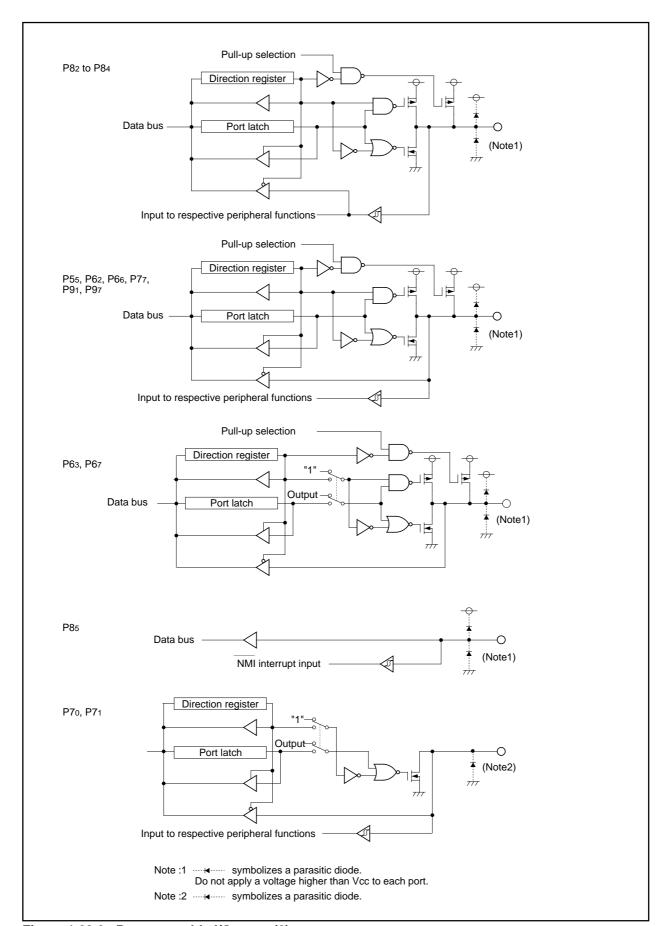
Figure 1.23.2. Programmable I/O ports (2)
