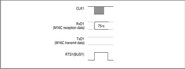
Figure 1.31.12. Timing for disabling the lock bit
