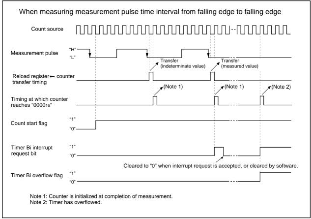
Figure 1.17.20. Operation timing when measuring a pulse period
