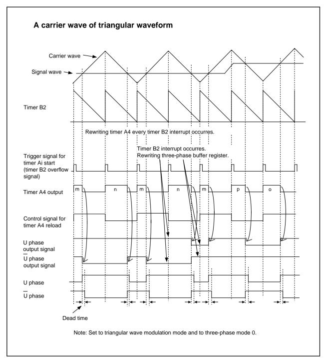
Figure 1.18.7. Timing chart of operation (2)
