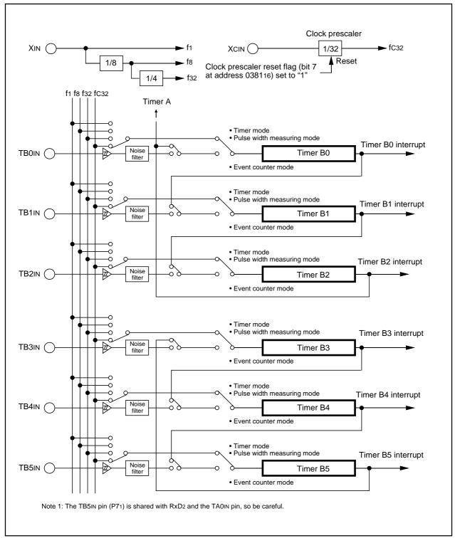
Figure 1.17.2. Timer B block diagram
