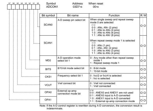
Figure 1.20.2. A-D converter-related registers (1)
