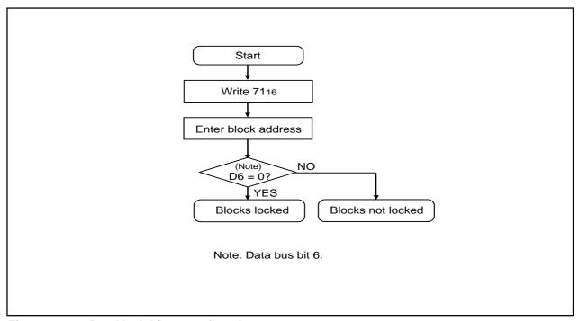
Figure 1.29.7. Read lock bit status flowchart
