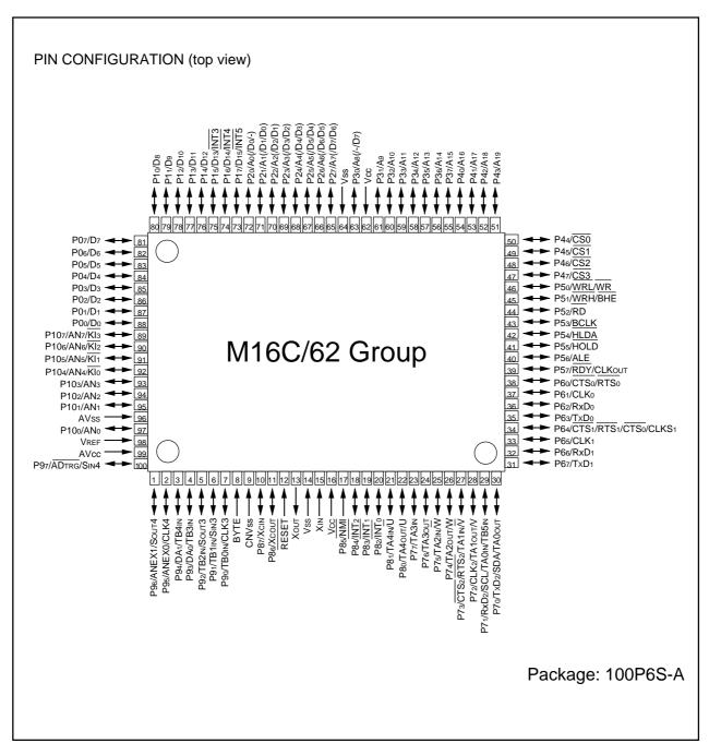
Figure 1.1.1. Pin configuration (top view)
