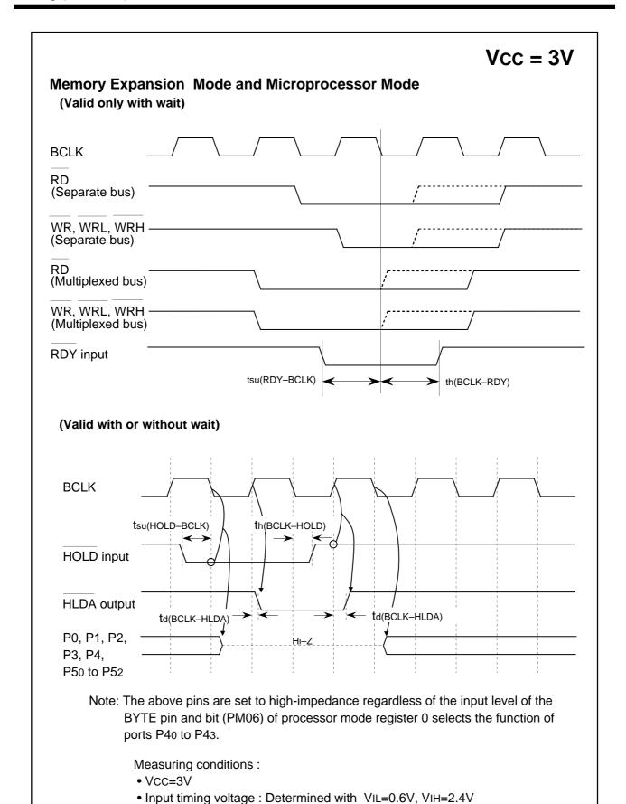
Figure 1.26.8. Vcc=3V timing diagram (2)
