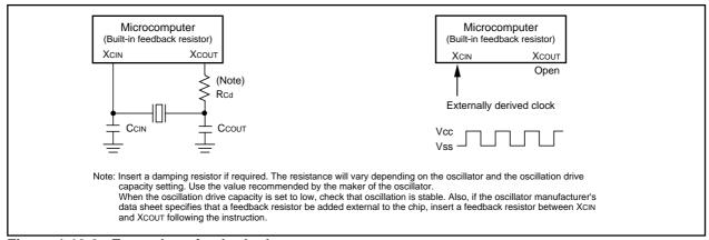
Figure 1.13.2. Examples of sub-clock
