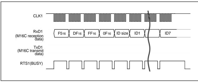
Figure 1.31.16. Timing for the ID check
