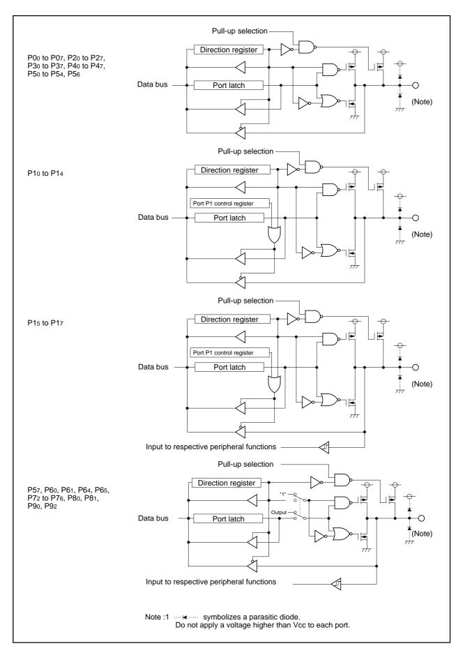
Figure 1.23.1. Programmable I/O ports (1)
