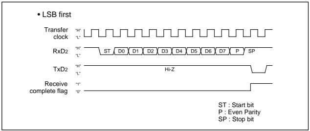
Figure 1.19.23. Output timing of the parity error signal
