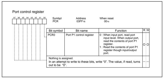
Figure 1.23.9. Port control register
