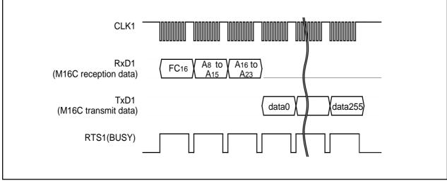
Figure 1.31.15. Timing for boot area output
