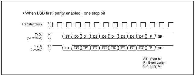
Figure 1.19.20. Timing for switching serial data logic
