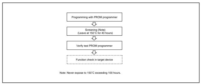
Figure 1.24.1. Programming and test flow for One Time PROM version
