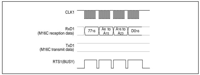
Figure 1.31.9. Timing for the lock bit program
