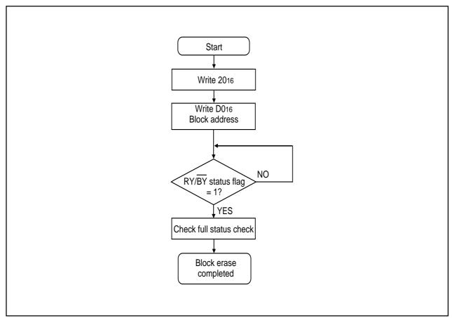
Figure 1.29.5. Block erase flowchart
