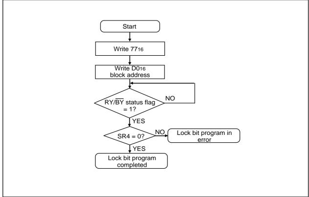
Figure 1.29.6. Lock bit program flowchart
