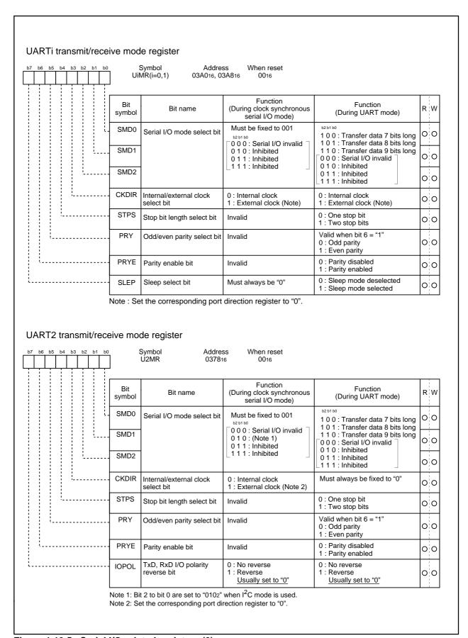
Figure 1.19.5. Serial I/O-related registers (2)
