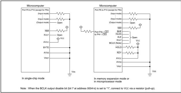
Figure 1.23.10. Example connection of unused pins
