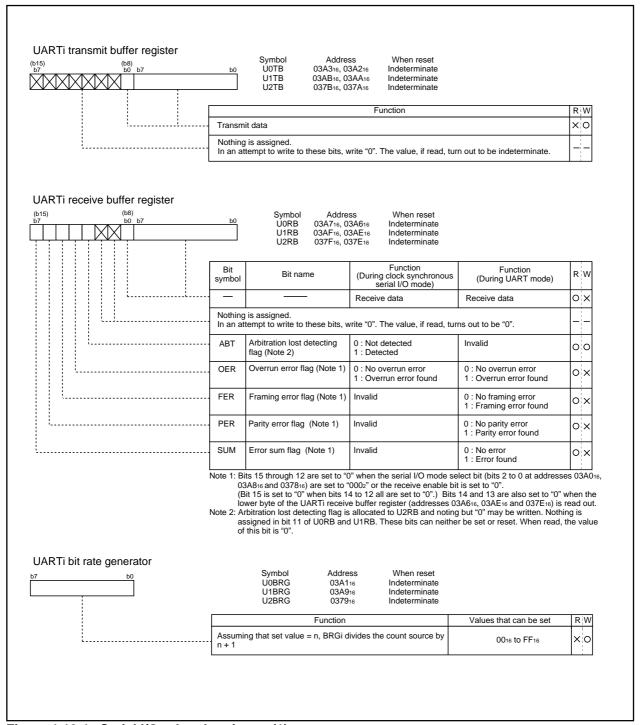
Figure 1.19.4. Serial I/O-related registers (1)
