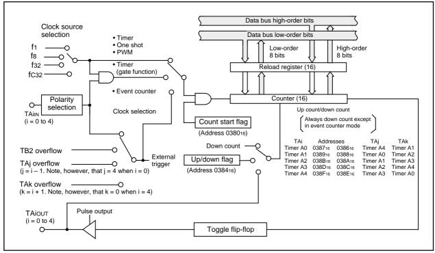
Figure 1.17.3. Block diagram of timer A
