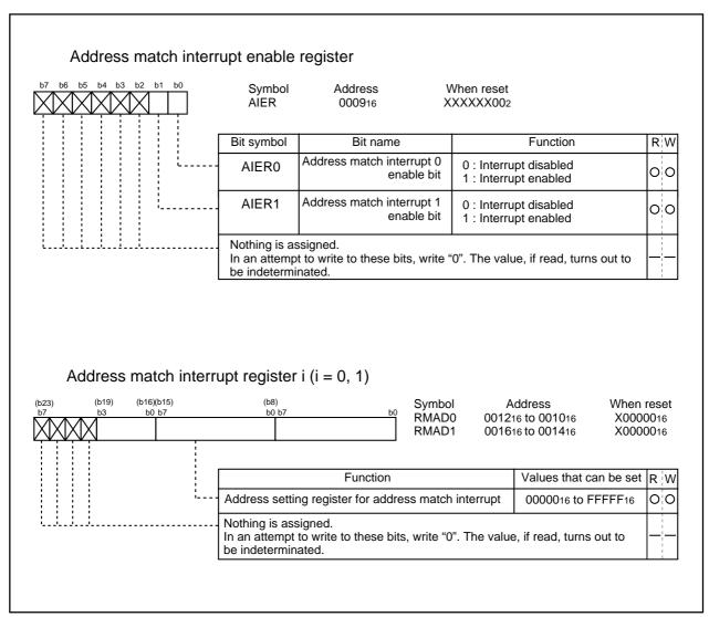
Figure 1.14.12. Address match interrupt-related registers
