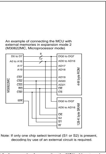
Figure 1.8.6. An example of connecting the MCU with external memories in expansion mode 2
