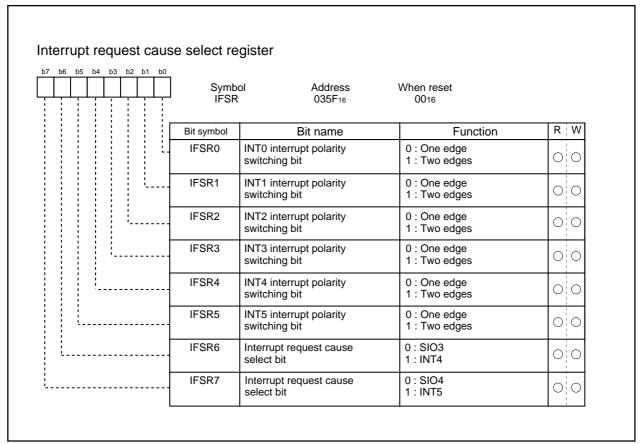
Figure 1.14.10. Interrupt request cause select register
