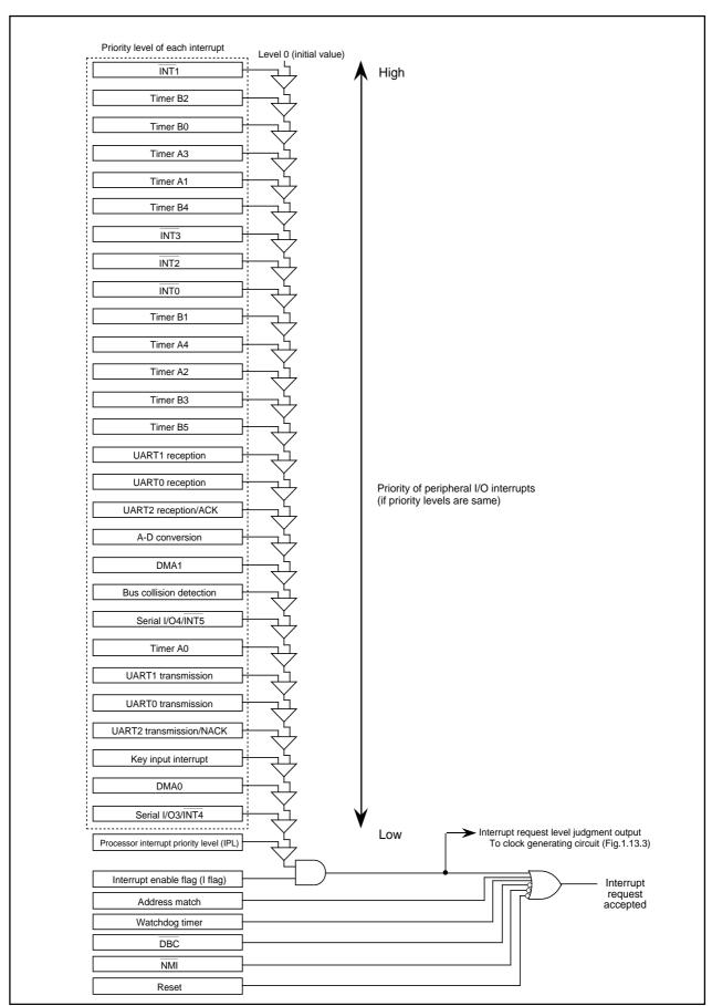
Figure 1.14.9. Maskable interrupts priorities (peripheral I/O interrupts)
