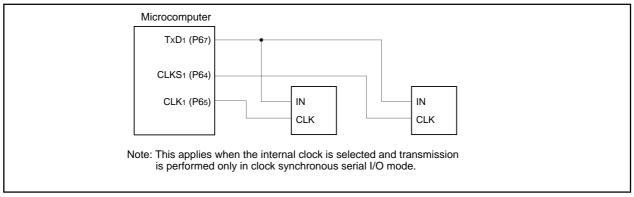
Figure 1.19.13. The transfer clock output from the multiple pins function usage
