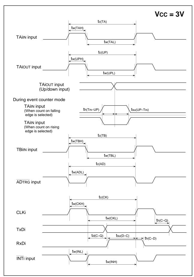
Figure 1.26.7. Vcc=3V timing diagram (1)
