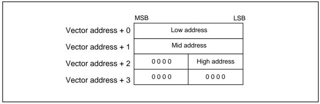
Figure 1.14.2. Format for specifying interrupt vector addresses
