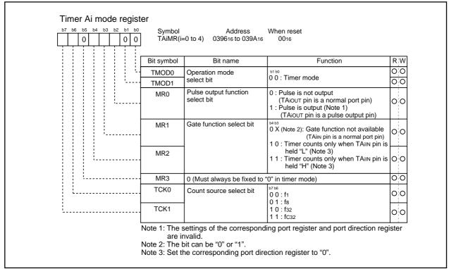
Figure 1.17.7. Timer Ai mode register in timer mode
