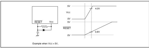
Figure 1.6.1. Example reset circuit
