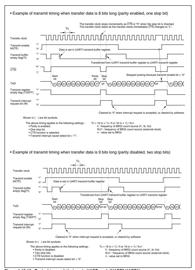
Figure 1.19.16. Typical transmit timings in UART mode(UART0,UART1)
