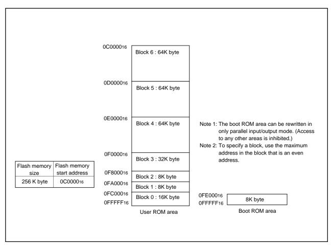
Figure 1.28.1. Block diagram of flash memory version
