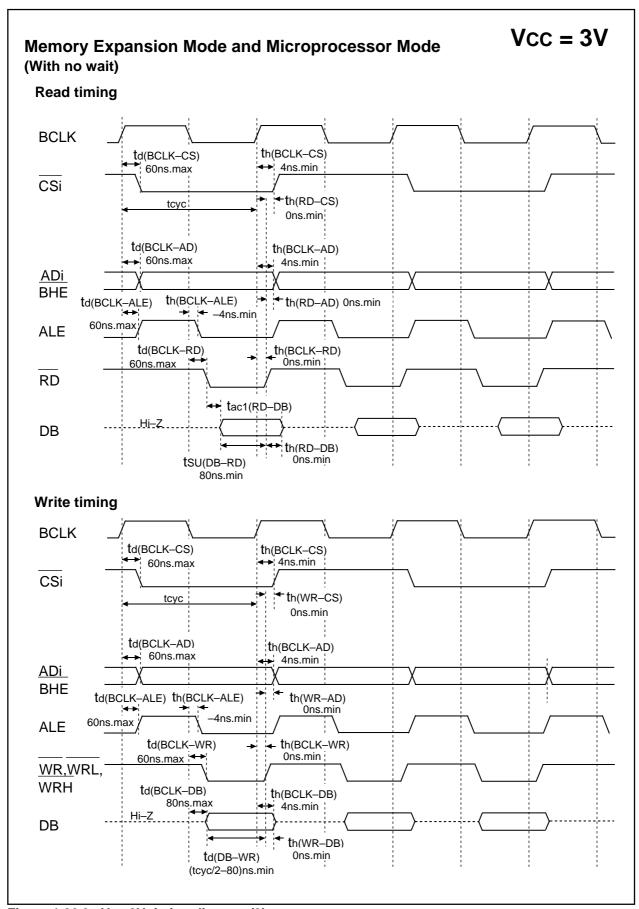
Figure 1.26.9. Vcc=3V timing diagram (3)
