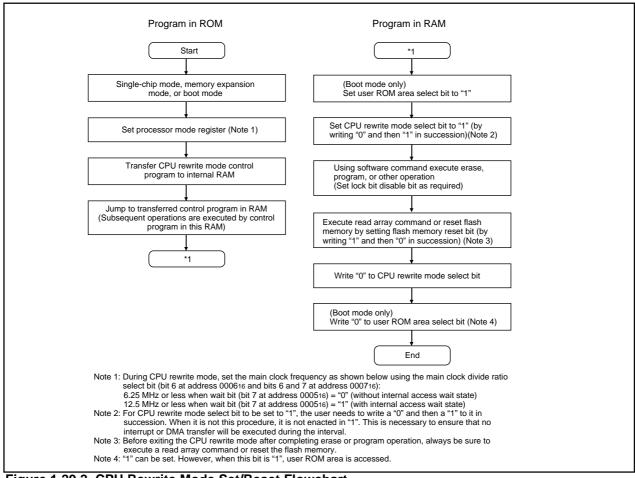
Figure 1.29.2. CPU Rewrite Mode Set/Reset Flowchart
