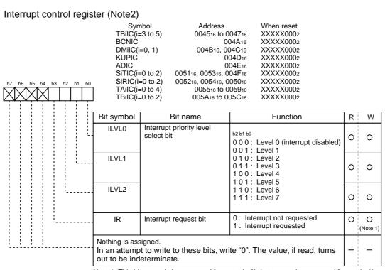
Note 1: This bit can only be accessed for reset (= 0), but cannot be accessed for set (= 1). Note 2: To rewrite the interrupt control register, do so at a point that dose not generate the interrupt request for that register. For details, see the precautions for interrupts.
