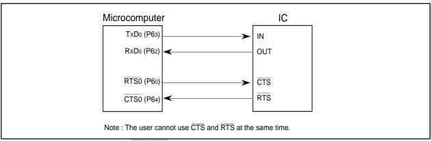
Figure 1.19.19. The separate CTS/RTS pins function usage
