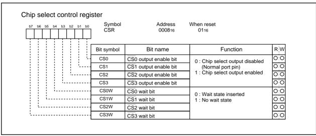
Figure 1.12.1. Chip select control register
