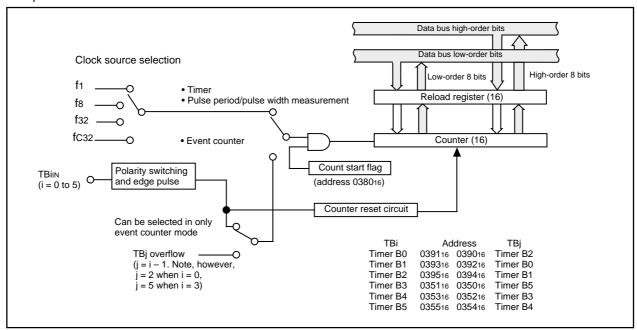
Figure 1.17.14. Block diagram of timer B
