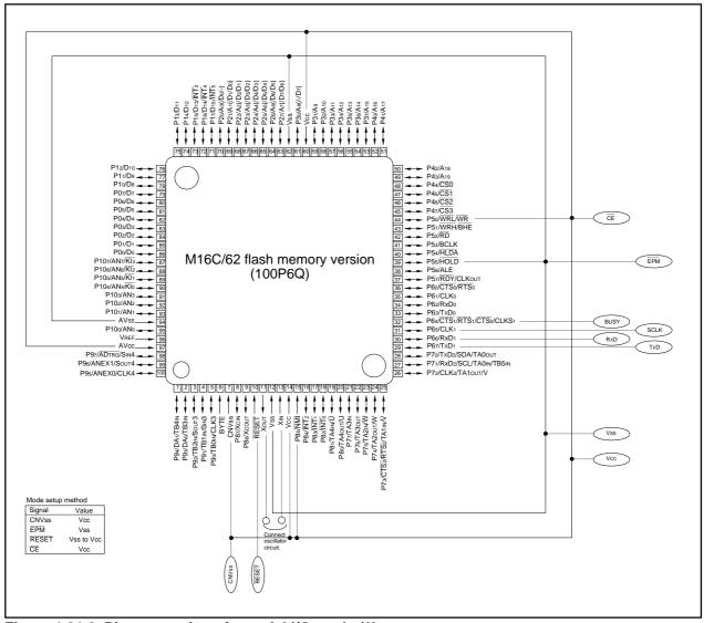
Figure 1.31.2. Pin connections for serial I/O mode (2)
