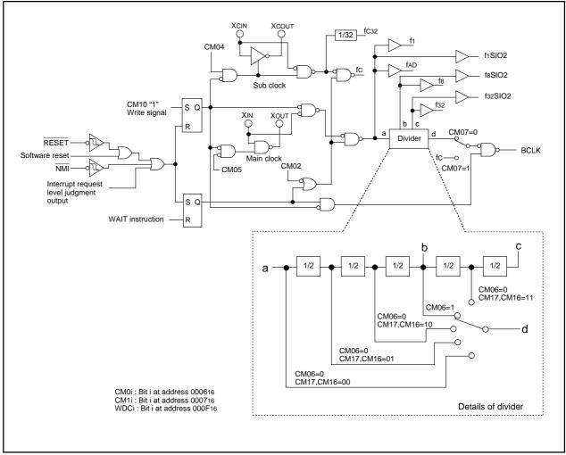
Figure 1.13.3. Clock generating circuit
