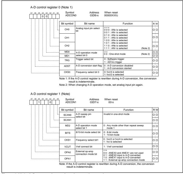
Figure 1.20.4. A-D conversion register in one-shot mode
