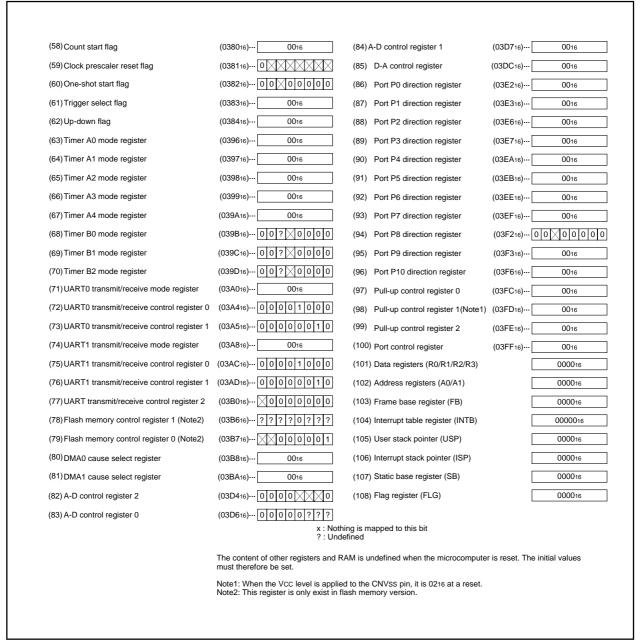
Figure 1.6.4. Device's internal status after a reset is cleared
