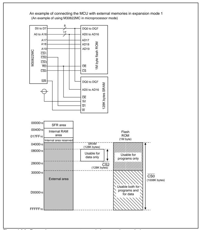
Figure 1.8.3. External memory connect example in expansion mode 1
