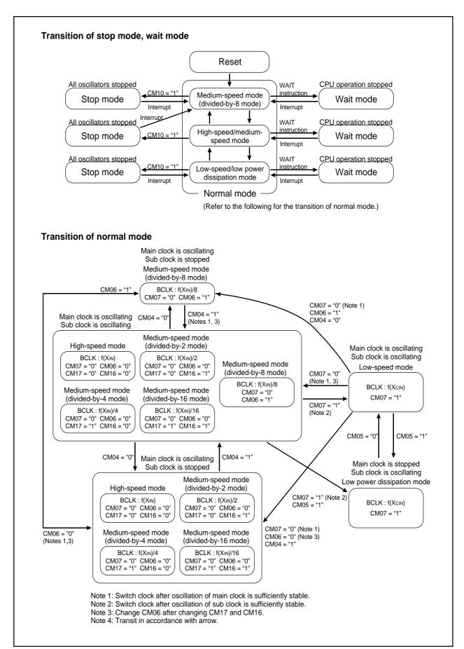
Figure 1.13.5. State transition diagram of Power control mode
