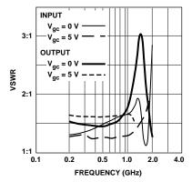
Figure 6. Input and Output VSWR vs. Frequency,  $V_{gc}$  = 0–5 V.
