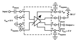
\* Optional: For Single-Ended Output operation, Pin 7 may be left unterminated (no C  $_{block}$  or 50  $\Omega)$
