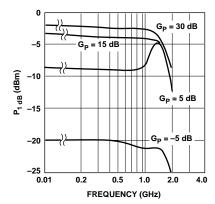
Figure 4. P<sub>1 dB</sub> vs. Frequency.
