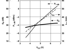
Figure 2. Power Gain and  $P_{1\ dB}$  at 0.5GHz and  $I_{CC}$  vs. Bias Voltage with  $V_{gc}=0\ V.$
