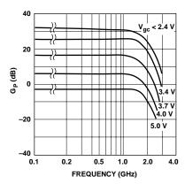
Figure 1. Typical Variable Gain vs. Frequency.
