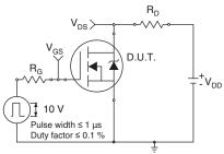
Fig. 10a - Switching Time Test Circuit
