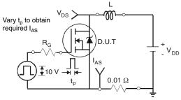
Fig. 12a - Unclamped Inductive Test Circuit
