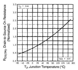
Fig. 4 - Normalized On-Resistance vs. Temperature
