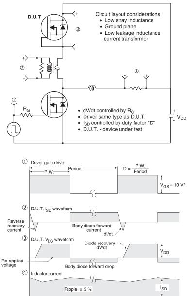
Peak Diode Recovery dV/dt Test Circuit
