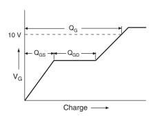
Fig. 13a - Basic Gate Charge Waveform
