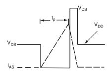
Fig. 12b - Unclamped Inductive Waveforms
