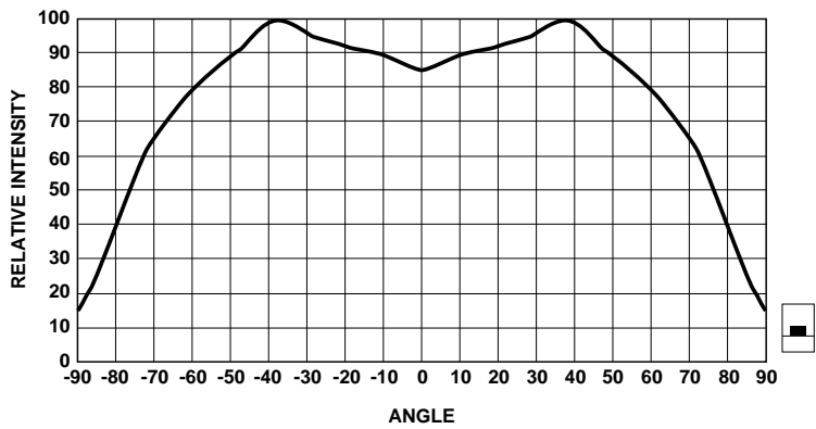
Figure 6. Relative Intensity vs. Angle for HSMx-C120.
