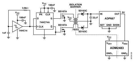
Figure 30. Isolated Power Supply Circuit
