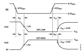
Figure 12. Receiver Enable/Disable Timing
