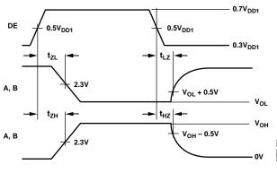
Figure 11. Driver Enable/Disable Timing
