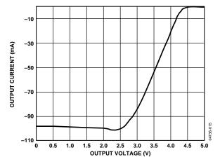
Figure 15. Output Current vs. Driver Output High Voltage
