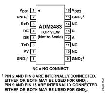
Figure 2. Pin Configuration
