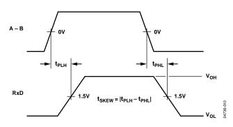
Figure 10. Receiver Propagation Delay
