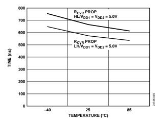
Figure 20. Receiver Propagation Delay vs. Temperature
