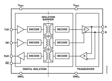
Figure 26. ADM2483 Digital Isolation and Transceiver Sections
