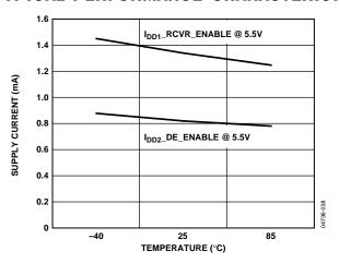
Figure 13. Unloaded Supply Current vs. Temperature
