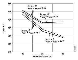
Figure 19. Driver Propagation Delay vs. Temperature
