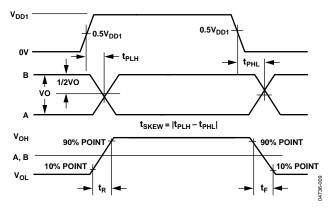
Figure 9. Driver Propagation Delay, Rise/Fall Timing
