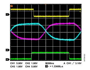
Figure 21. Driver/Receiver Propagation Delay High to Low
