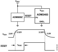
Figure 29. Driving PV with ADM809Z
