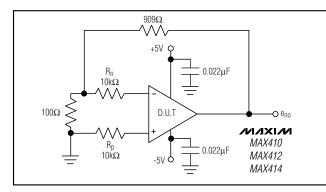
Figure 5. Current-Noise Test Circuit
