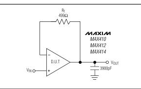
Figure 6a. Voltage Follower Circuit with 3900pF Load
