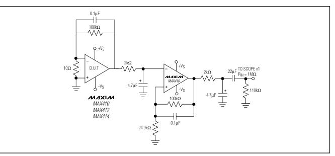
Figure 3. 0.1Hz to 10Hz Voltage Noise Test Circuit
