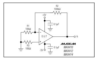
Figure 1. Total Noise vs. Source Resistance Example
