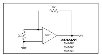
Figure 2. Voltage-Noise Density Test Circuit
