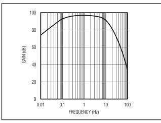
Figure 4. 0.1Hz to 10Hz Voltage Noise Test Circuit, Frequency Response
