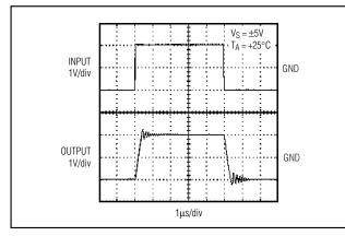
Figure 6b. Driving 3900pF Load as Shown in Figure 6a
