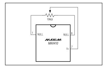
Figure 9. MAX410 Offset Null Circuit
