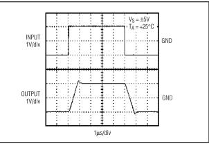
Figure 7b. Driving a 0.015 $\mu$ F Load with a 10 $\Omega$  Isolation Resistor
