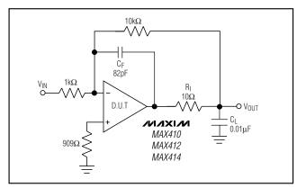
Figure 8. Capacitive-Load Driving Circuit with Loop-Enclosed Isolation Resistor
