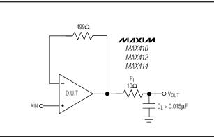
Figure 7a. Capacitive-Load Driving Circuit
