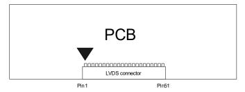
Note2. Please leave this pin unoccupied. It can not be connected by any signal (Low/GND/High)
