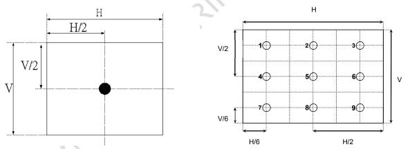
5. Viewing angle is the angle at which the contrast ratio is greater than 10. The angles are determined for the horizontal or x axis and the vertical or y axis with respect to the z axis which is normal to the LCD surface. For more information see FIG3.
