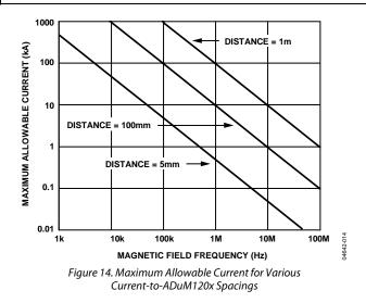
Note that, at combinations of strong magnetic fields and high frequencies, any loops formed by PCB traces can induce sufficiently large error voltages to trigger the threshold of succeeding circuitry. Care should be taken in the layout of such traces to avoid this possibility.
