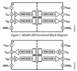
Figure 2. ADuM1201 Functional Block Diagram
