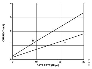
Figure 10. Typical ADuM1200 V<sub>DD2</sub> Supply Current vs. Data Rate for 5 V and 3 V Operation
