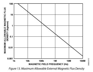
For example, at a magnetic field frequency of 1 MHz, the maximum allowable magnetic field of 0.2 kgauss induces a voltage of 0.25 V at the receiving coil. This is about 50% of the sensing threshold and does not cause a faulty output transition. Similarly, if such an event occurs during a transmitted pulse (and has the worst-case polarity), it reduces the received pulse from >1.0 V to 0.75 V—still well above the 0.5 V sensing threshold of the decoder.
