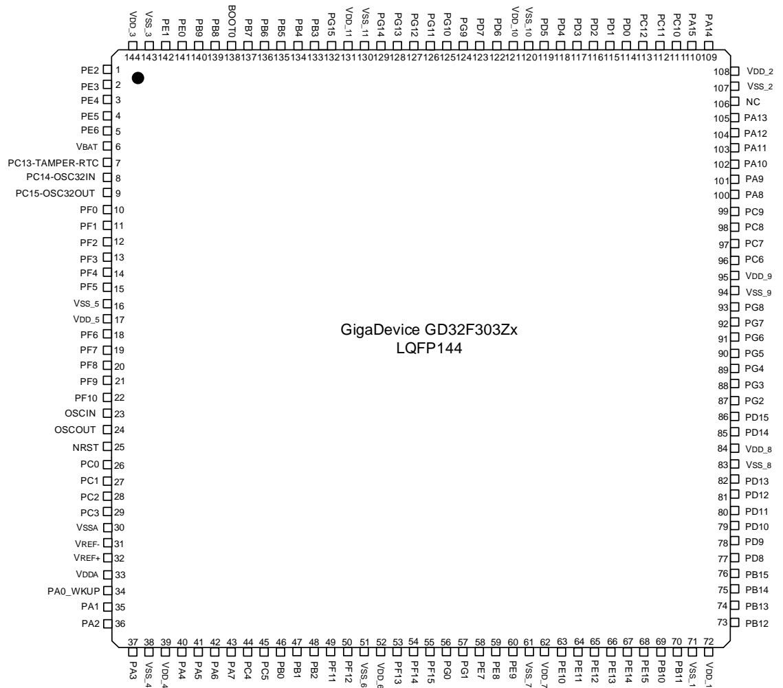
Figure 2-2. GD32F303Zx LQFP144 pinouts
