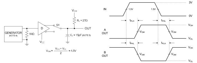
Fig. 4. Driver Propagation Delay
