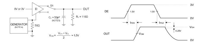
Fig. 5. Driver Enable and Disable Times, Output High
