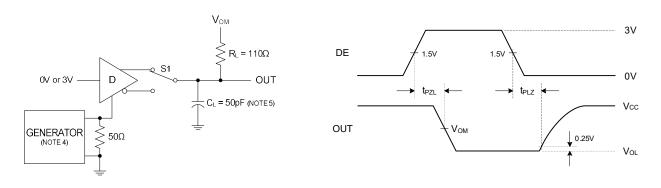
Fig. 6. Driver Enable and Disable Times, Output Low
