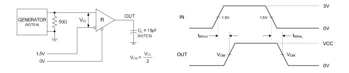
Fig. 7. Receiver Propagation Delay
