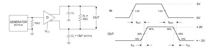
Fig. 3. Driver Differential Output Delay and Transition Times
