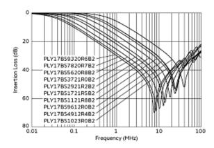
Common Mode Insertion Loss-Frequency Characteristics
