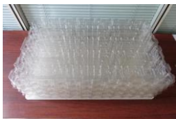
8. Stack 8layers PET tray as the method mention above (7tray+1dummy tray)
